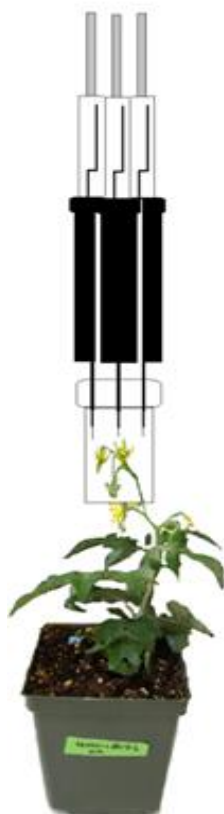
Figure 3.2. Experimental setup for the in vivo sampling of Micro-Tom flowers. VOCs were allowed to accumulate in the vial for 24 h prior to the introduction of three SPME fibers (extraction time 20 min).
