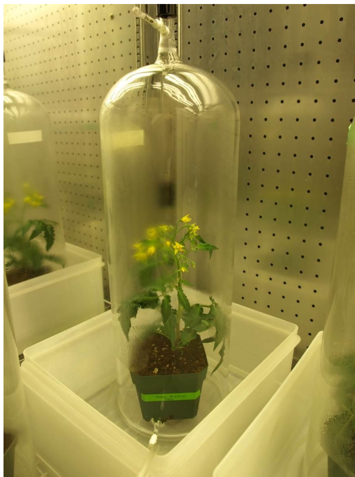
Figure 2.17. Glass chamber for the dynamic headspace (DHS) collection of volatiles. Every chamber contained a pot with one Micro-Tom tomato plant at flowering stage.
