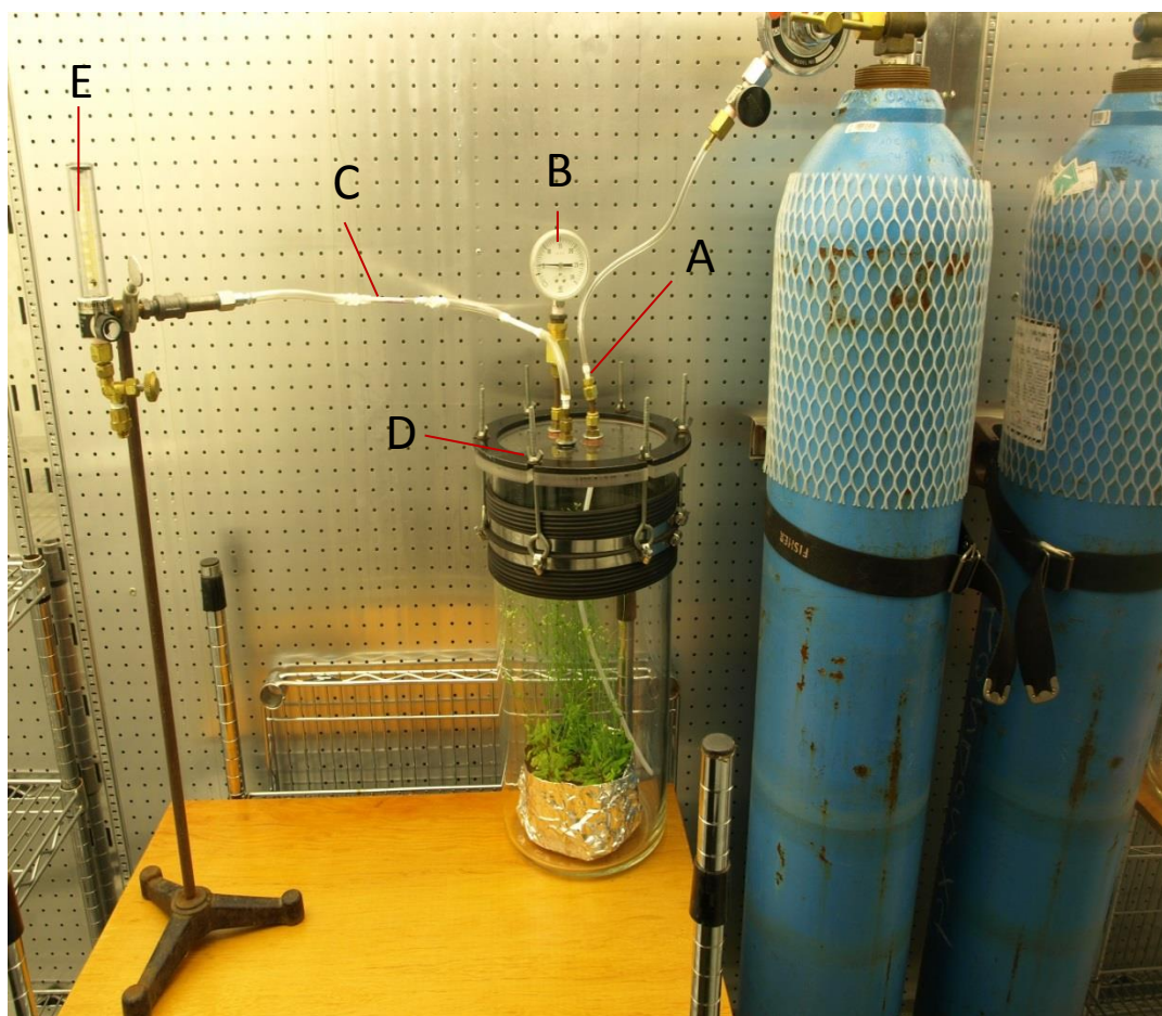
Figure A2 Cylindrical glass chamber (48 cm height X 28 cm diameter) with a compressed air tank used initially to test collection of plant volatiles. Inlet (A), gauge to monitor HS pressure (B), air outlet tubing with a cartridge to trap volatiles (C), and flowmeter (E).
