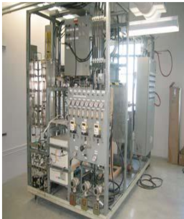
Figure A11 Fluidized bed reactor at the Institute for Chemicals and Fuels from Alternative Resources (ICFAR) from the University of Western Ontario. The reactor was used to obtain bio-oil from tomato plant residue biomass by pyrolysis process.
