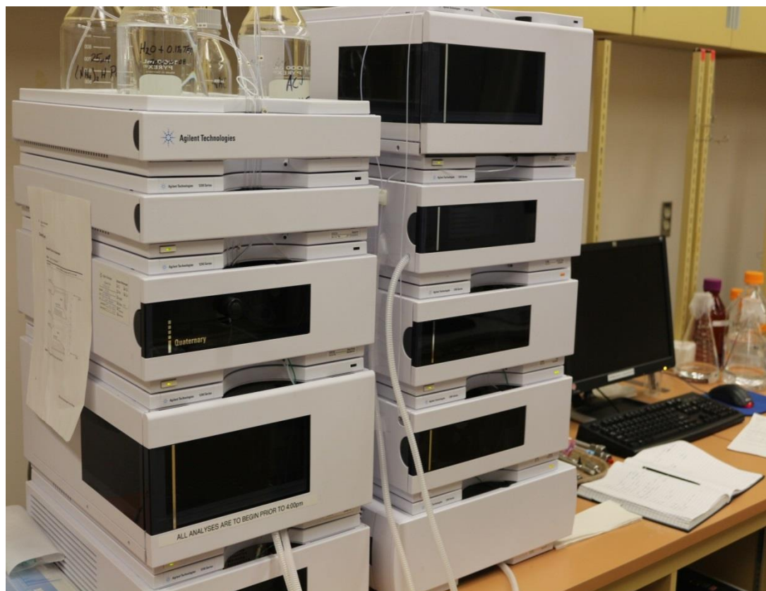
Figure A12 LC separation and fraction collection of the most active hexane sub-fraction, Fraction a, was performed on an Agilent 1200 Series liquid chromatographic system Agilent Technologies Canada Inc.
