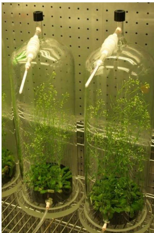
Figure 2.4. Two glass chambers for the dynamic headspace (DHS) collection of volatiles. Every chamber contains a pot with a set of seven to eleven Arabidopsis thaliana ecotype-0 plants at flowering stage.
